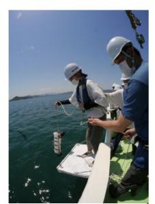
Water sampling by Van Dorm Sampler.
