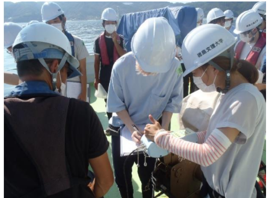
Measuring the water temperature, salt content, oxygen concentration, photon, etc. at each water depths.
