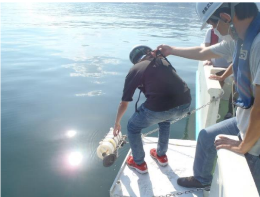
Sampling the waters at the required depths by a Van Dorm Sampler.
